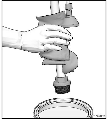
4. Place fluid intake in flushing fluid. Use water for water base paint and mineral spirits for oil-based paint. Place drain tube in waste pail.
