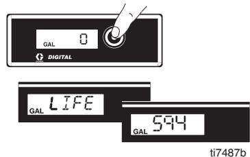
6. To change pressure units (psi, bar, or MPa), press and hold display button for eight seconds until desired units appear. Selection of bar or MPa changes gallons to Liters x10.
