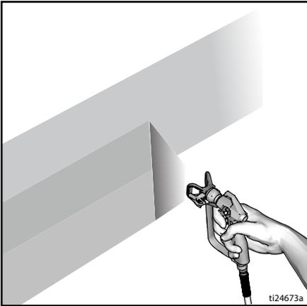
4. Trigger gun after moving. Release trigger before stopping. For additional spraying information, see separate gun manual.
