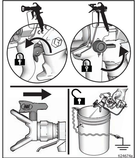
2. Engage trigger lock. Return Spray Tip to original position. Disengage trigger lock and continue spraying.
