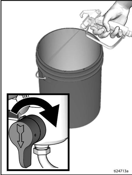
6. Turn pressure control to Fast Flush operate until the pump runs steady and flushing fluid appears in the waste pail.
