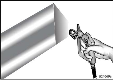
2. Use smaller tip size if pressure adjustment cannot eliminate heavy edges.
