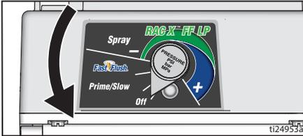
3. Turn ON/OFF switch to **ON** position.
