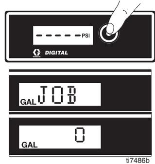
5. Press and hold display button to reset to zero, or short press button to move to Lifetime Gallons (or Liters x10).
